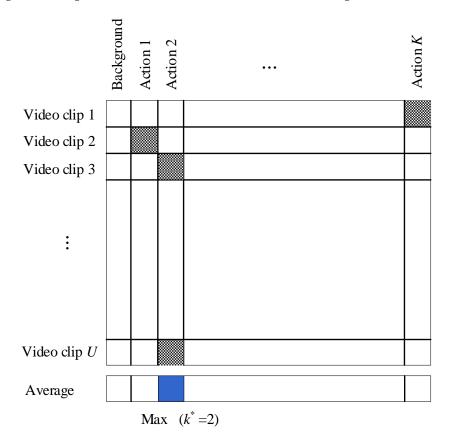
**Figure 3.** The diagrammatic sketch on the determination of video category  $k^*$  from video clips.
