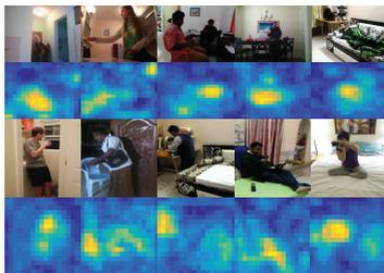
Figure 5: Global video-clip representation visualization, extracted after layer “conv6” of backbone network.
