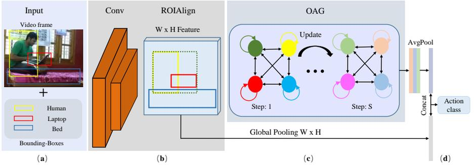
Figure 2: OAGN overview. **(a)** OAGN takes video frames and ground truth human/objects bounding-boxes as inputs. **(b)** RoIAlign [14] produces region-based features according to the bounding-boxes (including the union of bounding-boxes). **(c)** Graph nodes are iteratively updated in  $S$  steps, and they are initialized with extracted feature maps within respective bounding-boxes. **(d)** After practical convergence, updated nodes and video features are concatenated for action prediction.
